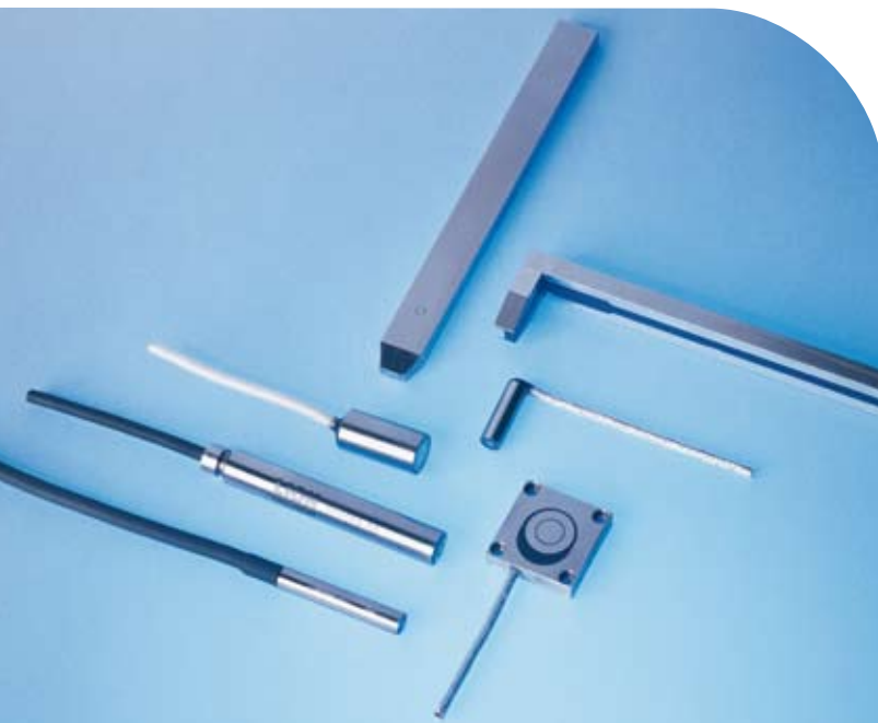
Various different types and sizes of capacitive sensors for measuring distance very precisely
